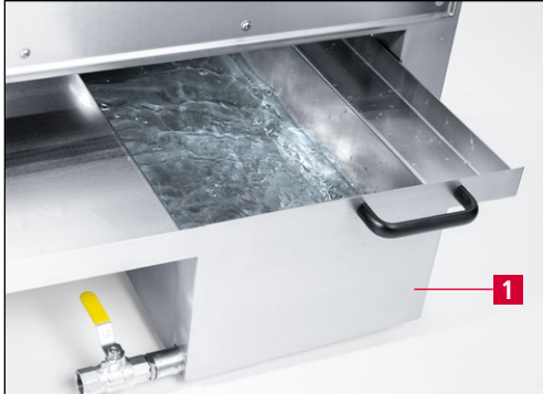
Figure 9-21 Replacing the coolant water
