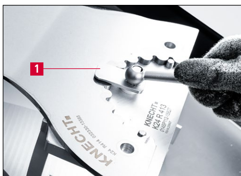
Figure 7-6 Locking the knife
