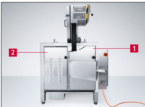
Figure 3-8 Doors polishing and deburring unit
