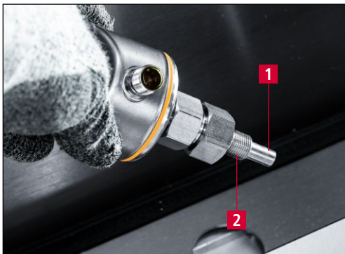
Figure 9-9 Cleaning the flow monitor
