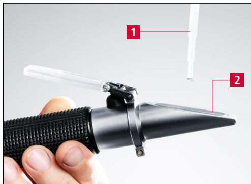
Figure 9-22 Measuring the cooling lubricant concentration
