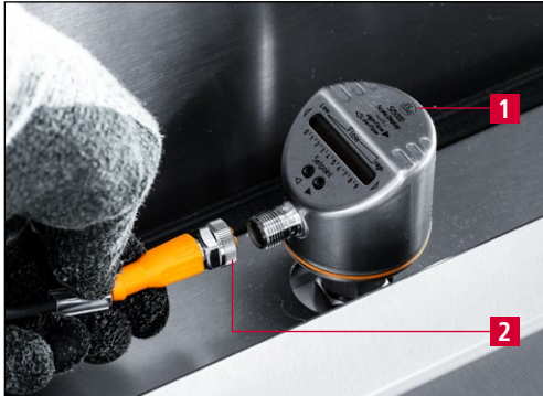
Figure 9-8 Unplugging the flow monitor
