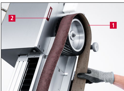
Figure 7-61 Replacing the wet-grinding belt
