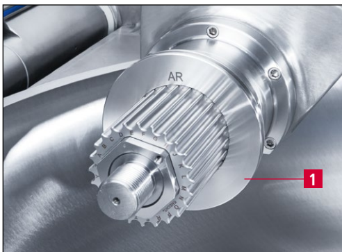
Figure 5-1 Installing the initial ring (AR)
