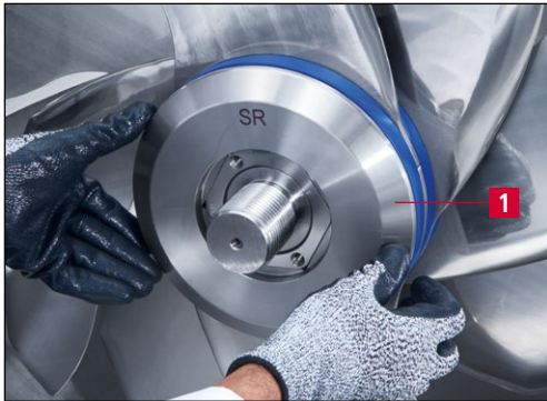
Figure 5-10 Installing the end ring (SR)
