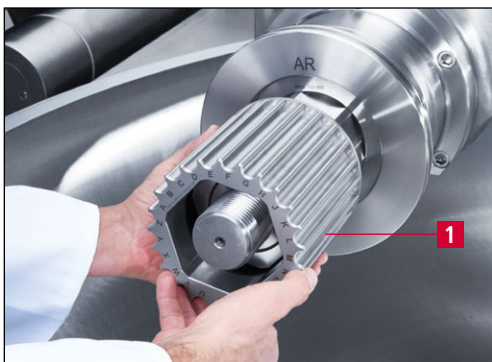
Figure 5-2 Installing the profile sleeve
