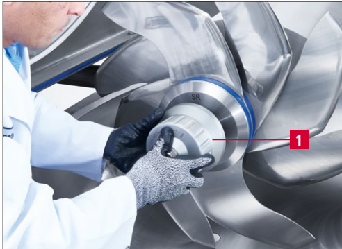
Figure 5-12 Installing the MCF 100 Mechanical Spring Clamping Nut
